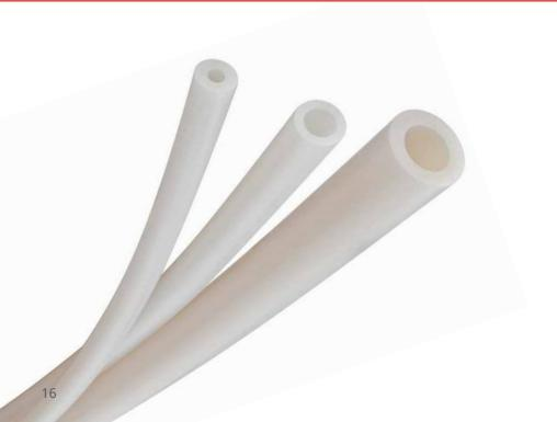
PTFE-reinforced fluoroelastomer tubing which handles nearly all aggressive chemicals, including organic solvents such as methyl ethyl ketone, toluene and acetone. With 50 times longer life than other fluoroelastomers and pressures up to 4 bar.
