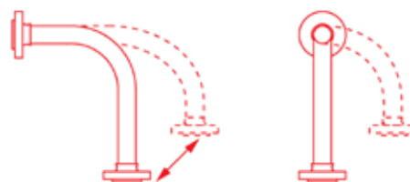
INCORRECT - Flexing movement takes place in 3 dimensions so torque is applied
