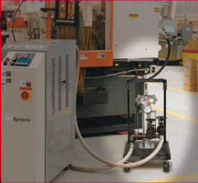
Portable version in-line with a Mokon HTF System, featuring the optional Delta P gauge.
