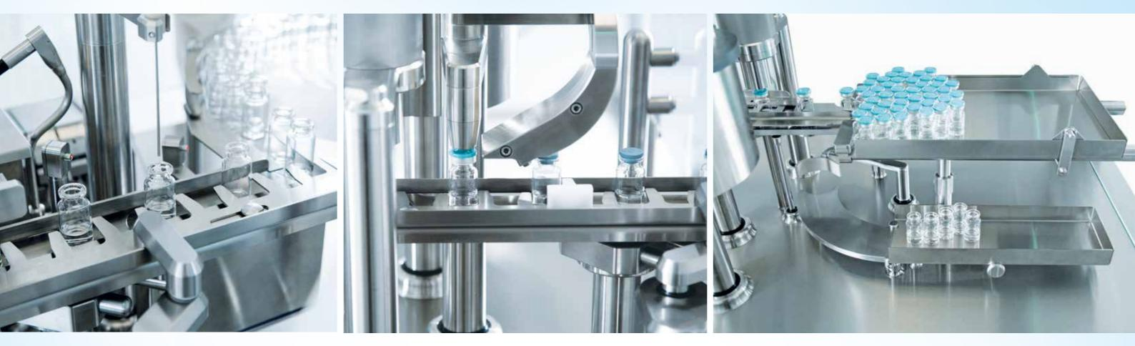
When supplied with in-line check weighing, the FPC60 offers unique dynamic prime, no intervention initial calibration and dynamic recalibration, meaning no waste in the batch start up process and confirmation every vial, from first to last, is filled within specification.
