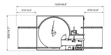
Dimensions in mm/inch. On FlexFeed20 and FlexFeed15 the infeed tray can easily be mounted on the front or on the left side of the machine.
